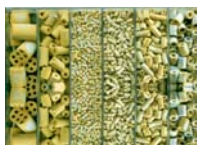
Vanadium pentoxide catalysts for sulfuric acid production
